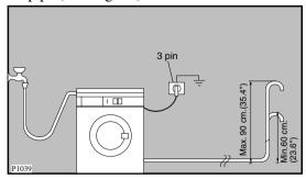
Make sure that it is designed in such a way, that the end of the drain hose cannot be covered with water. The drain hose may be extended to a maximum of 4 metres.
